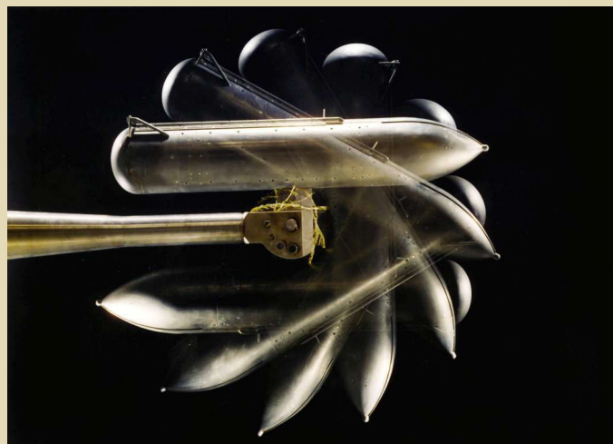
Aerodynamicists tumbled a scale model of the space shuttle's external tank to simulate the stress of reentry.
